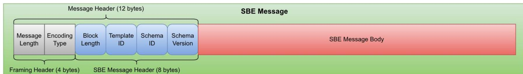
Framing Header is based on **Simple Open Framing Header (SOFH)**, but *MessageLength* field occupy only 2 bytes (support maximum message size of 16384 bytes): <https://www.fixtrading.org/standards/fix-sofh/>
