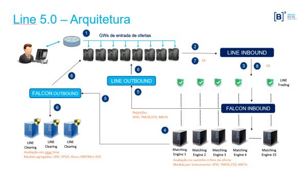
In this architecture, each trading engine has a single Trading Risk Center to control risk (affinity per engine). In it, the FIFO is guaranteed from LiNe. Additionally, the trading gateways, which currently make the routing of the offers to trading centers, will no longer do this, so that, as from the implementation of this project, the risk centers of the LiNe trading will start to route the offers to the trading centers.
